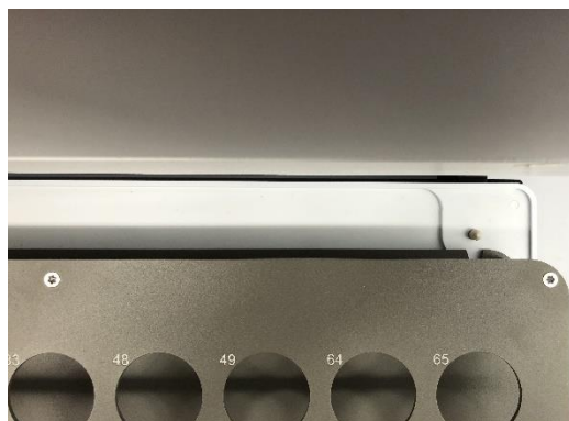
Fig. 22 and Fig. 23 Left and right groove of the inserted sample rack
