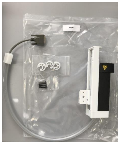
Fig. 3 Bag 2 with titration tower and tube clamps
