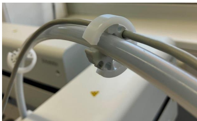
Fig. 17 Cable attached to the power supply via cable guide.
