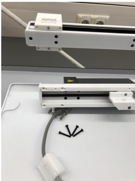
Fig. 7 and Fig. 8 Mounting the titration tower
