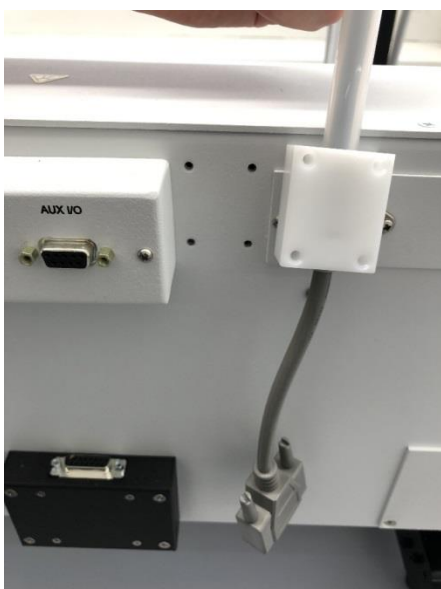
Fig. 9 and Fig. 10 Mounting the cable guide
