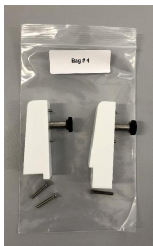
Fig. 5 Bag 4 with holders for titration heads
